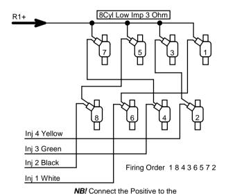
**Note!** Your firing order and piston numbers may differ from the examples. Determine which pistons move up and down together and wire them together. See also the manual for how to determine from the firing order which injectors must be grouped together.
